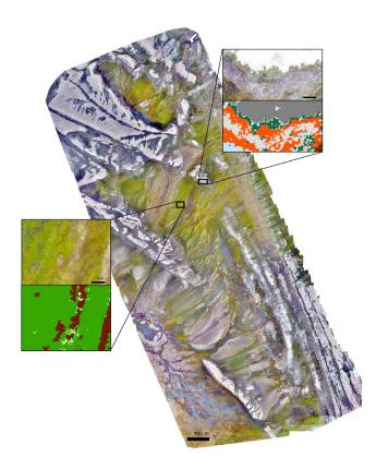
In COAT we focus on using the most efficient measurement method for each occasion, implementing new technologies and methods when needed. We collect aerial imagery using an eBeeX UAV and then use very precise differential GPS to ground-validate the imagery. This combined with field measurements provides a complementary dataset that reliably quantifies the goose activities and their impact on vegetation. Photo Isabell Eischeid / Norwegian Polar Institute
